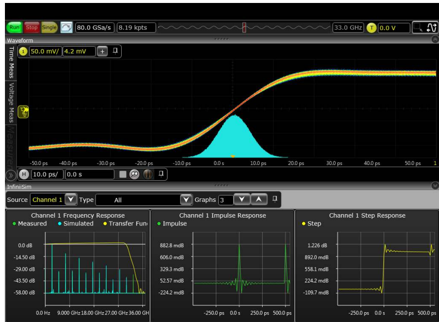
InfiniiSim renders the waveform through hardware acceleration.
