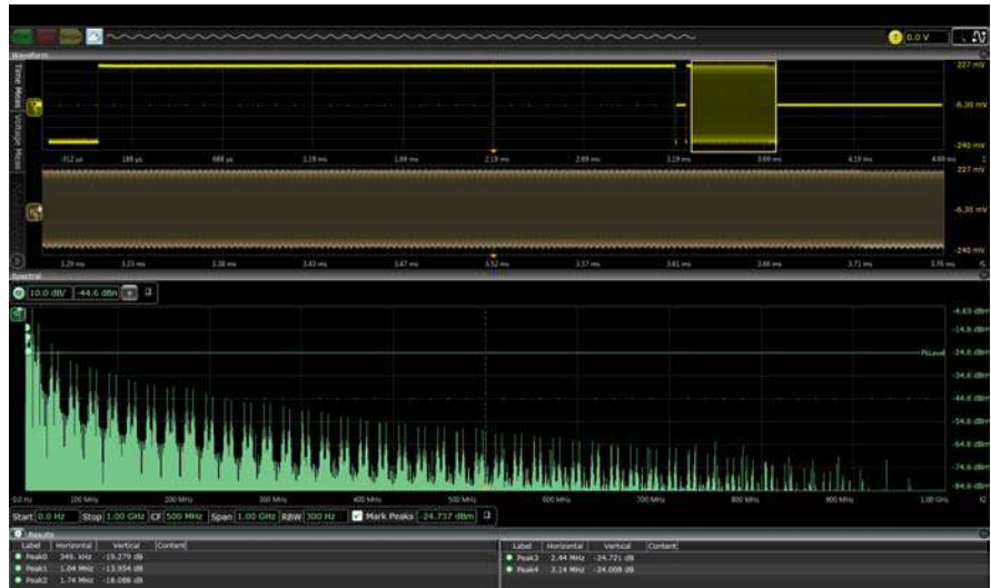
The Z-Series FFT quickly identifies peaks and has key controls such as span, start and stop, which make the oscilloscope behave more like a spectrum analyzer.
