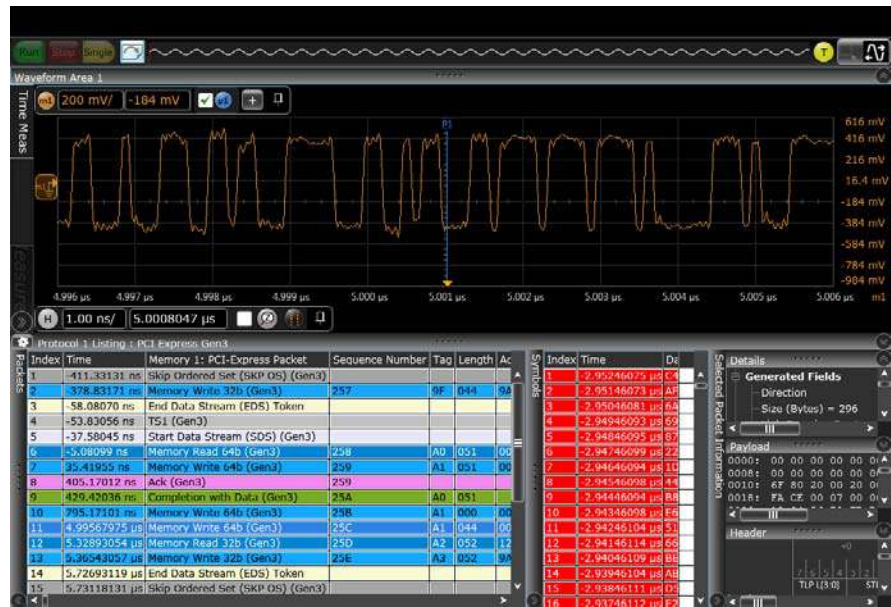
Z-Series decoding the PCI Express Gen 3 packets.
